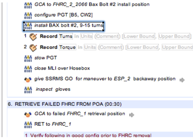
Figure 13: BAX bolt installation with required recording instructions
